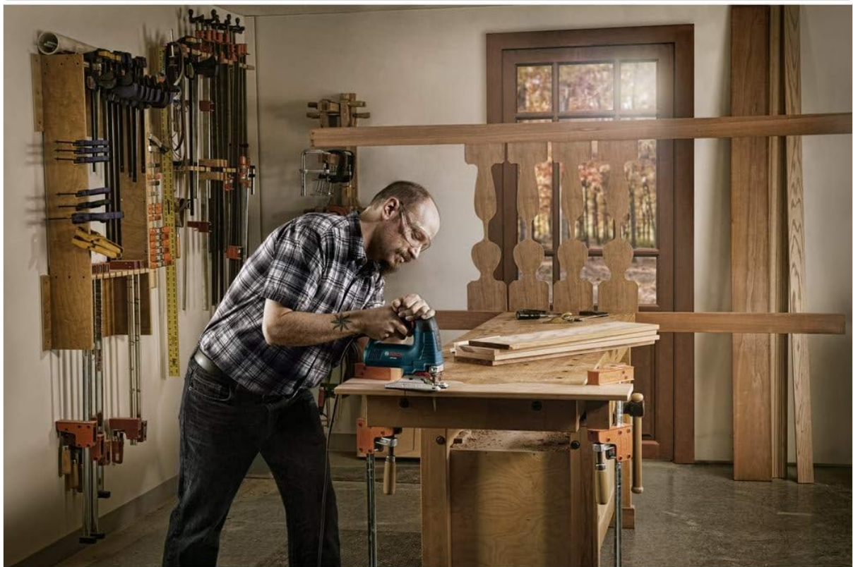
Image: A user demonstrating the application of a jigsaw blade for cutting, emphasizing the importance of securing the workpiece.
