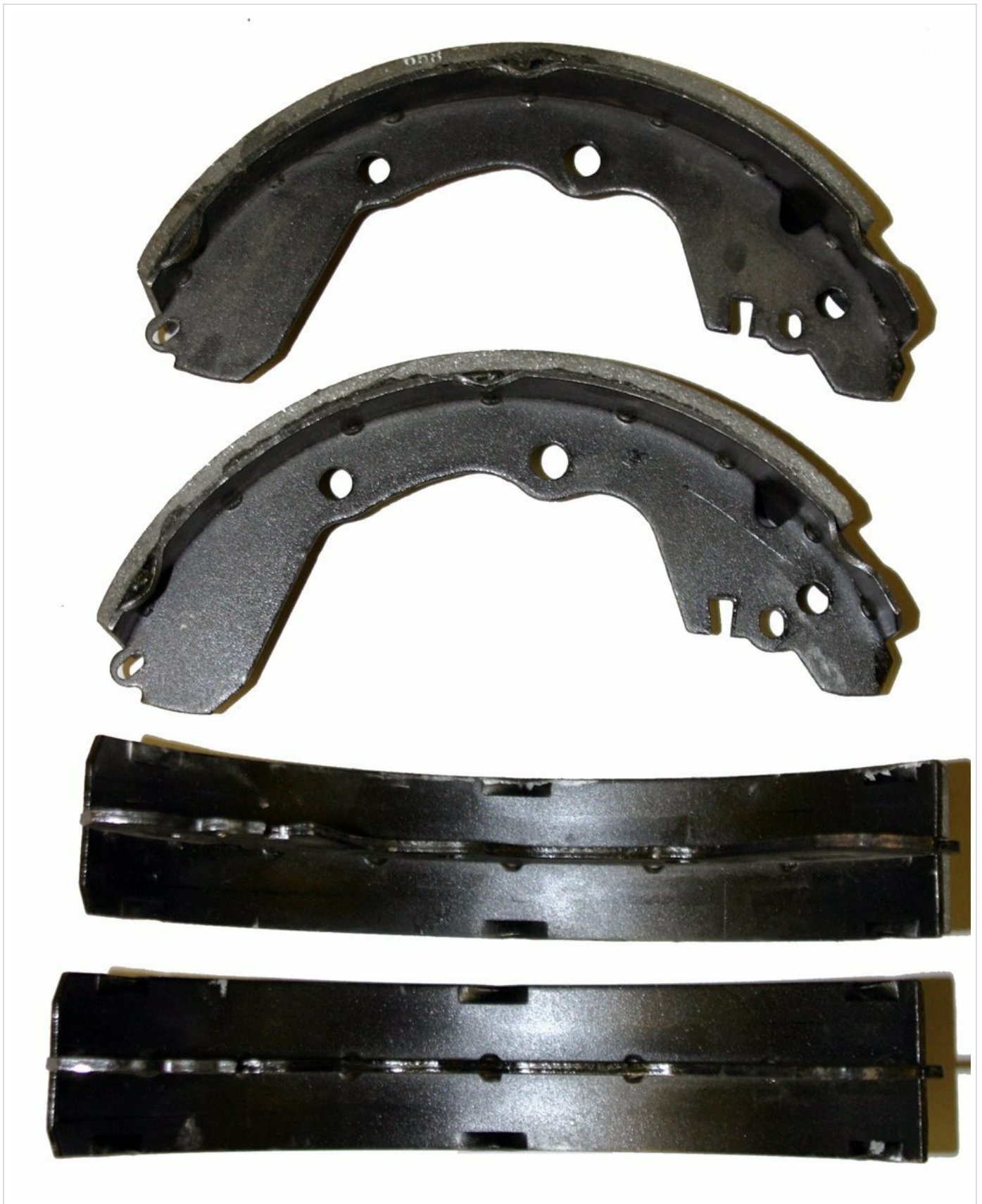
Figure 1: An example of the Monroe BX658 Bonded Brake Shoe. This image shows the brake shoe with its friction material and carbon steel backing plate, ready for installation.
