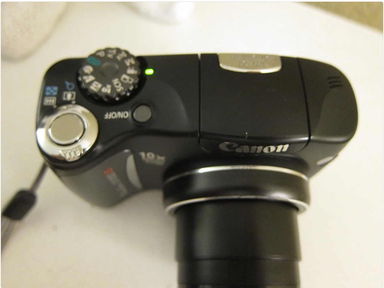
Figure 3: Top view of the Canon PowerShot SX100IS, highlighting the ON/OFF button and the Mode Dial for selecting shooting modes.
