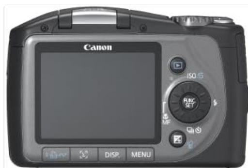
Figure 4: Rear view diagram of the Canon PowerShot SX100IS, illustrating the LCD screen and the arrangement of control buttons, including the control wheel and function buttons.
