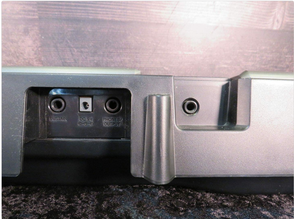
Image: Rear panel connections including DC 9V power input.
