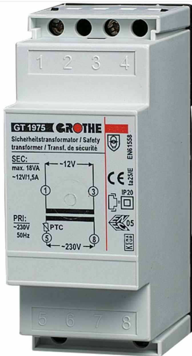
Figure 3.1: Front view of the Grothe 14101 Doorbell Transformer, showing the model number (GT 1975), electrical specifications (230V primary, 12V/1.5A secondary, 18VA max), safety certifications (CE, VDE, EN61558, IP20), and a detailed wiring diagram with terminal numbers.
