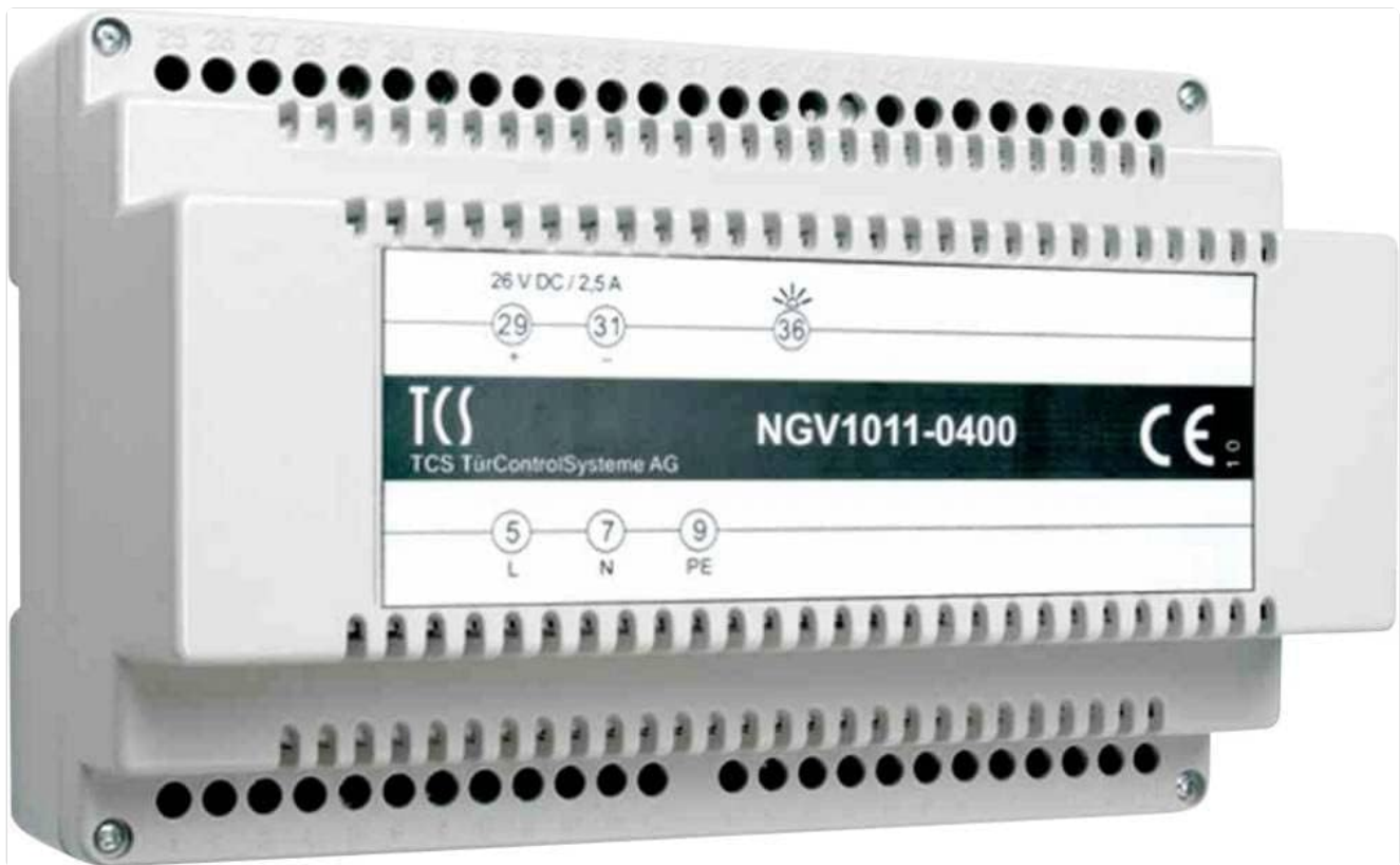
Figure 1: TCS NGV1011-0400 Intercom Accessory Control Unit. This image displays the TCS NGV1011-0400 intercom accessory control unit. The front panel features the TCS logo, model number NGV1011-0400, and CE marking. Terminal blocks are visible at the top and bottom for electrical connections. The label indicates an output voltage of 26 V DC / 2.5 A and AC input terminals L, N, PE.
