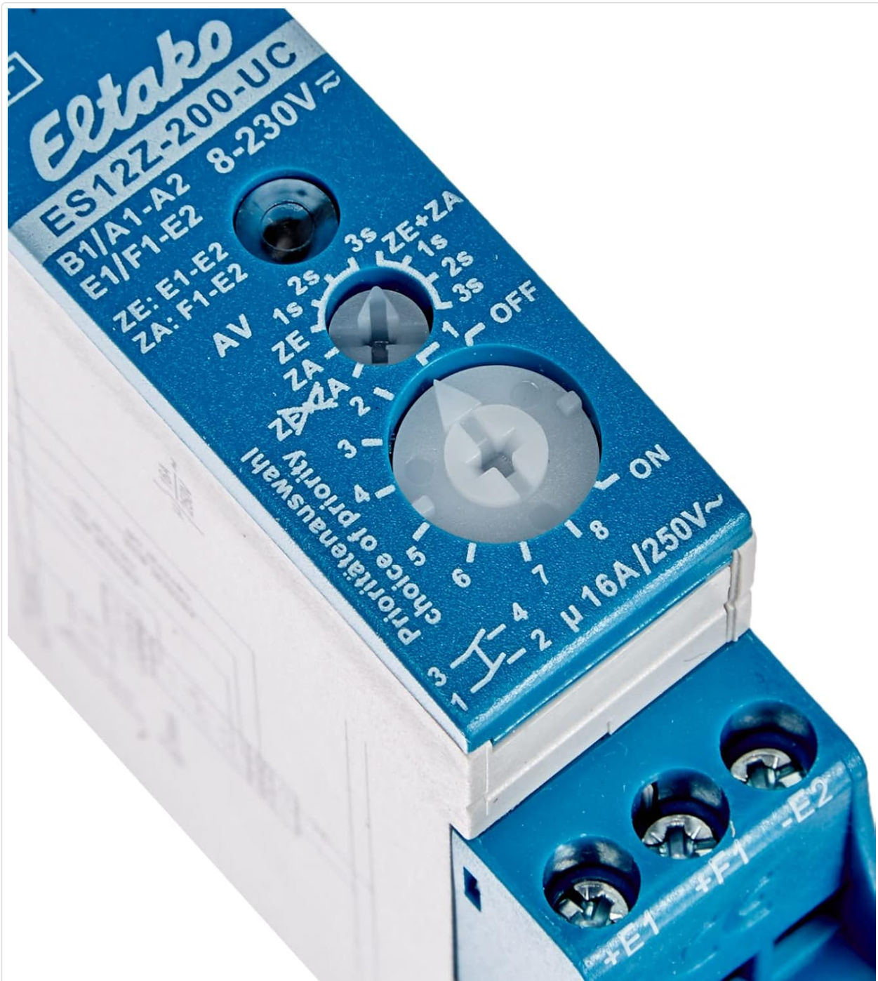
Image 2: Close-up view of the Eltako ES12Z-200 rotary switch. This switch allows users to select different priority levels for control inputs and configure the relay's response to power outages, such as switching off or maintaining its current state.
