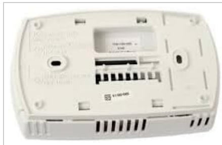
Figure 5.1: Rear view of the thermostat with the wallplate removed, showing wiring terminals.
