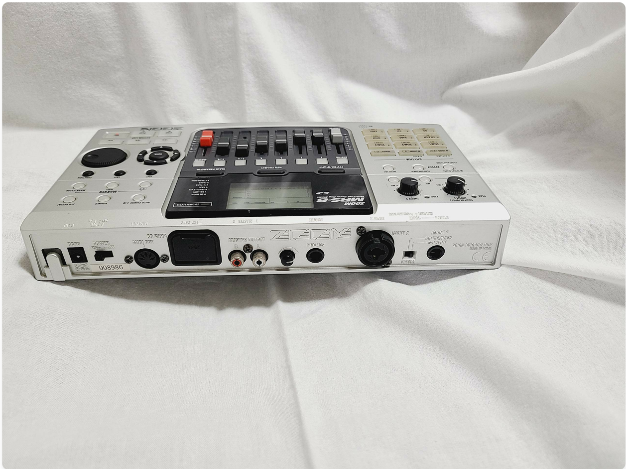
Rear view of the Zoom MRS8, displaying the various input and output ports including Hi-Z, XLR, RCA, Headphone, and MIDI.
