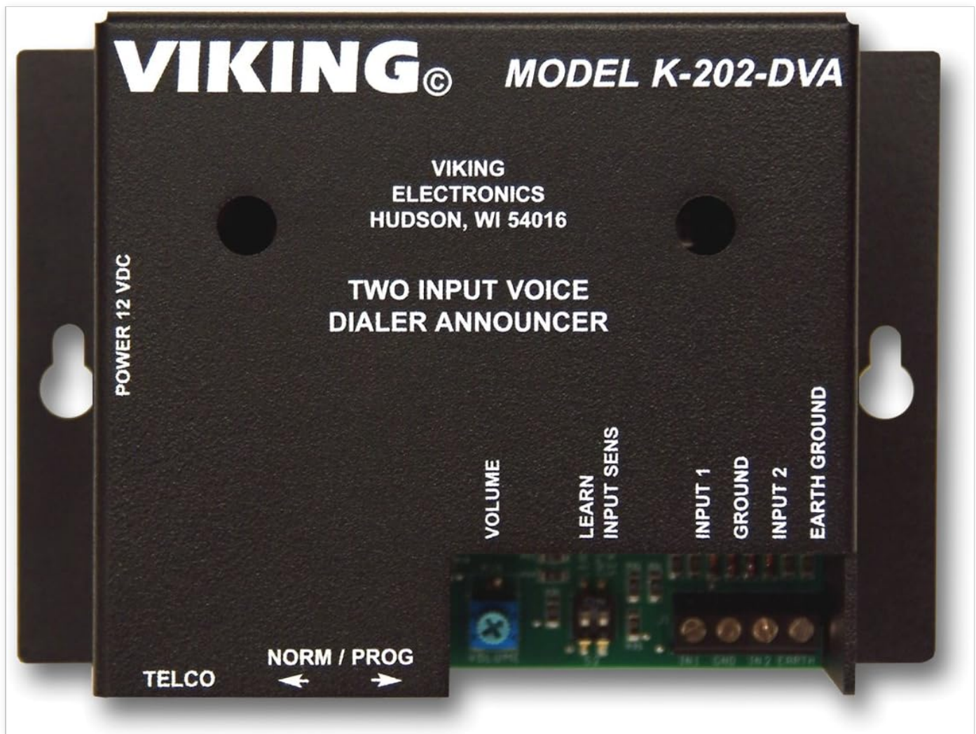
Figure 1: Front view of the Viking K-202-DVA showing power, TELCO, volume, input, and ground connections.
