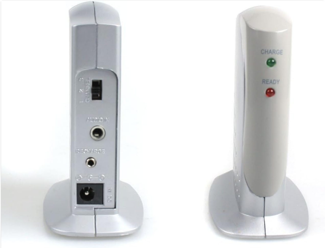
Image: Vivanco FMH 6050 Transmitter back view. This image displays the rear panel of the transmitter, showing the CHANNEL switch, AUDIO IN port, RECHARGE port, and DC IN power input.
