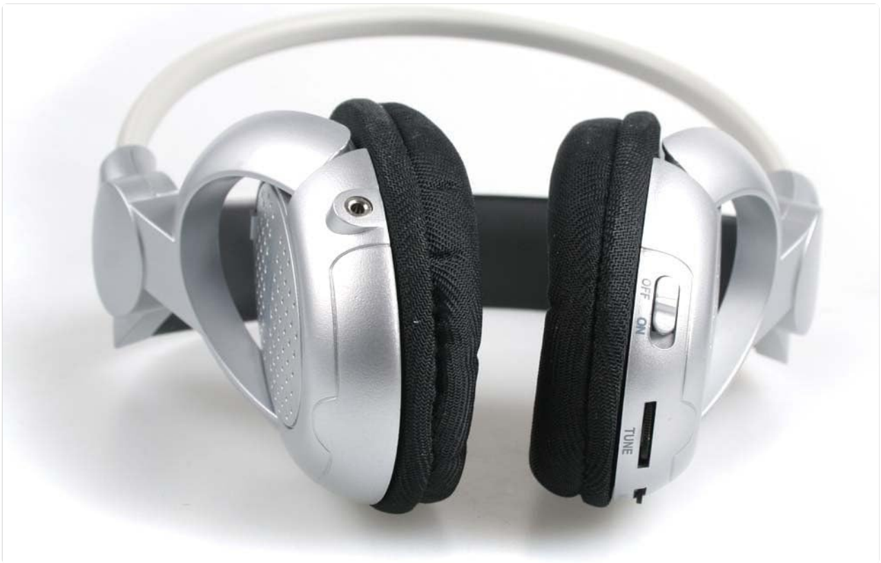
Image: Vivanco FMH 6050 Headphones front view. This image shows the right earcup with the ON/OFF switch and the TUNE button.
