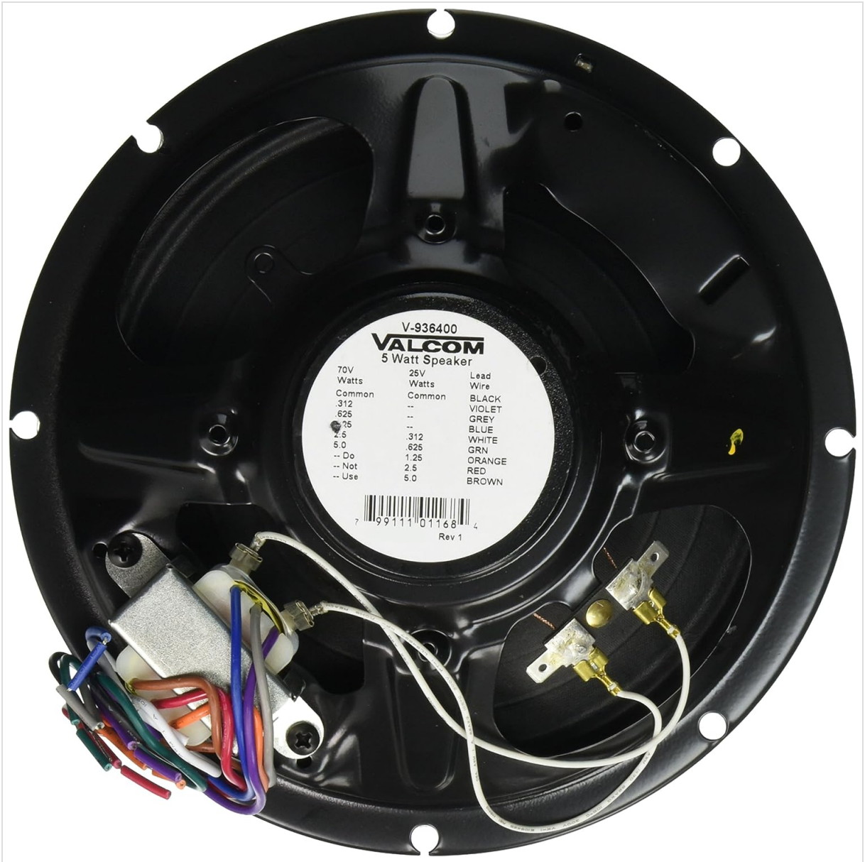
Image 5.1: Rear view of the Valcom V-936400 speaker, displaying the wiring terminals and the label detailing 70V and 25V tap settings with corresponding wire colors.
