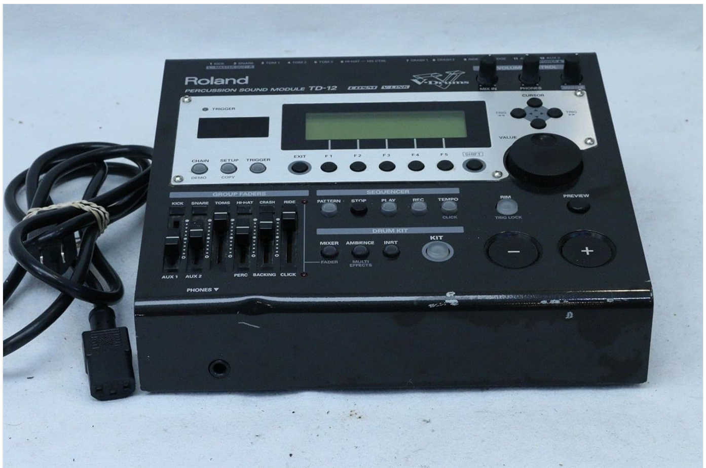
Figure 4.1: Front Panel of the TD-12 Module. This image shows the front interface of the Roland TD-12, featuring the main LCD display, navigation buttons (CHAIN, SETUP, TRIGGER, EXIT, F1-F5, SHIFT), a VALUE dial, VOLUME knob, MIX IN knob, PHONES jack, GROUP FADERS for KICK, SNARE, TOMS, HI-HAT, CRASH, RIDE, and dedicated buttons for MIXER, AMBIENCE, INIT, MULTI EFFECTS, DRUM KIT, SEQUENCER controls (PATTERN, STOP, PLAY, REC, TEMPO, CLICK), and +/- buttons.
