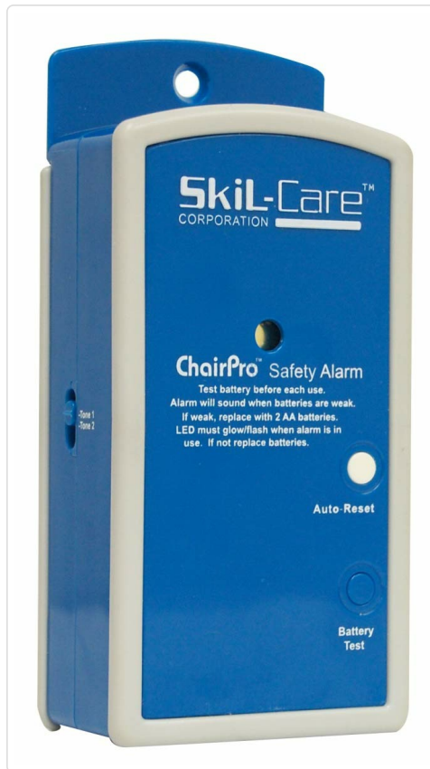
Figure 3.1: Skil-Care ChairPro Safety Alarm Unit. This image shows the main alarm unit with its front panel, including the Skil-Care logo, "ChairPro Safety Alarm" text, Auto-Reset button, Battery Test button, and an indicator light. The side of the unit shows "Tone 1" and "Tone 2" labels, indicating volume or tone settings.
