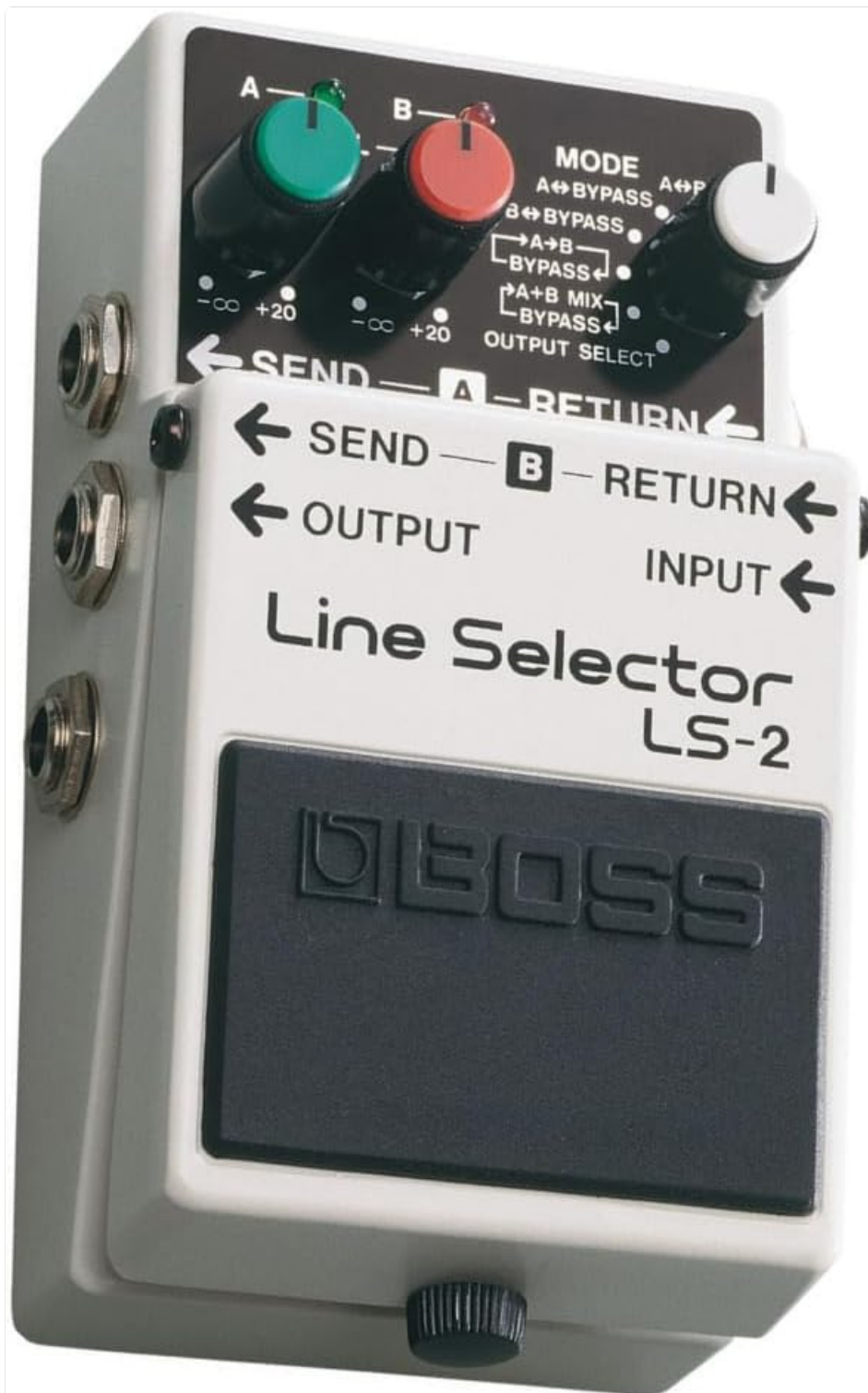
Figure 3.2: Side view of the BOSS LS-2 pedal, illustrating the various 1/4-inch audio jacks for input, output, and the two send/return loops.
