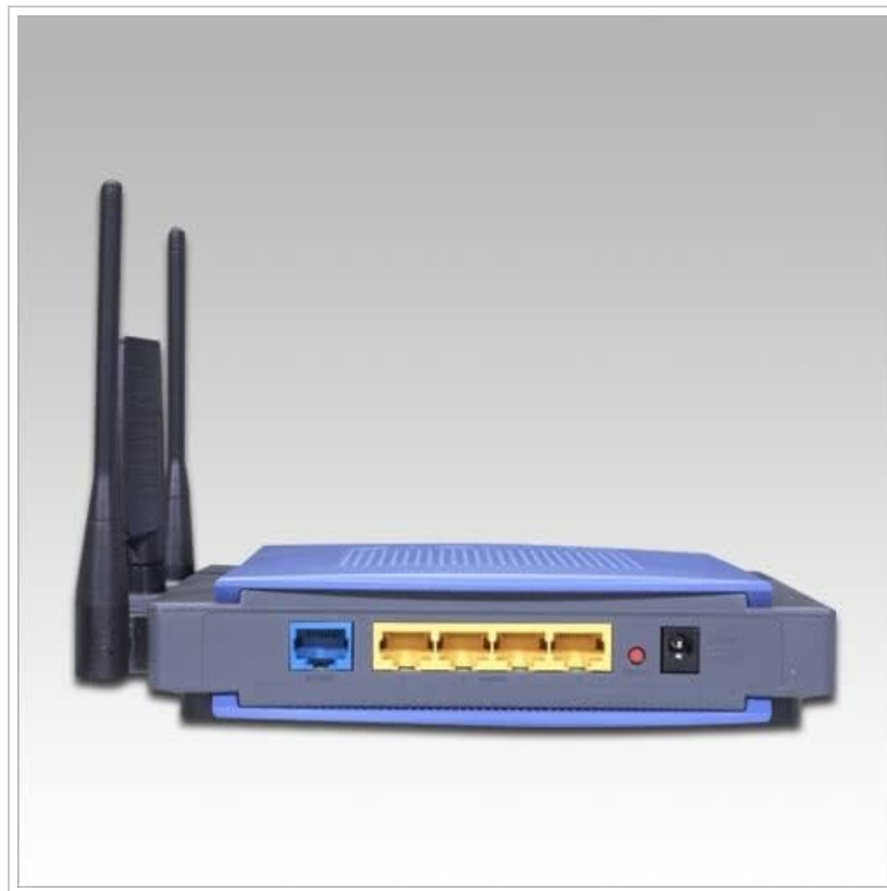
Figure 2: Rear panel of the Linksys WRT300N, illustrating the Internet (blue) and LAN (yellow) ports, along with antenna connections and power input.
