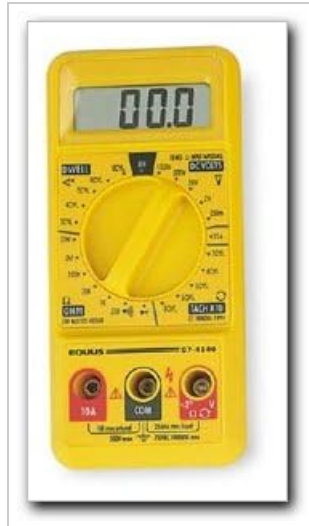
Figure 1: Front view of the Equus 4340 Digital Engine Analyzer. This image shows the digital display, the central rotary dial for function selection, and the three input jacks at the bottom for connecting test leads.
