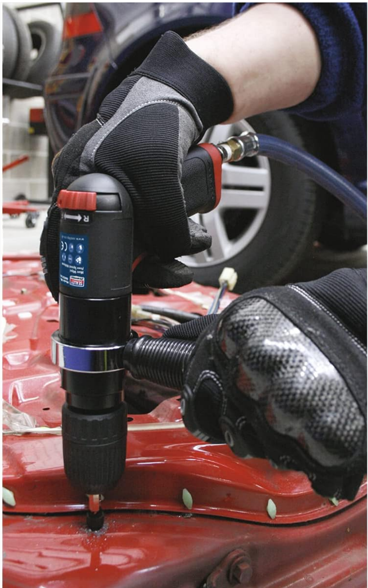
Figure 5.1: The Sealey SA621 Air Drill in operation, demonstrating its use for precision drilling in automotive applications.
