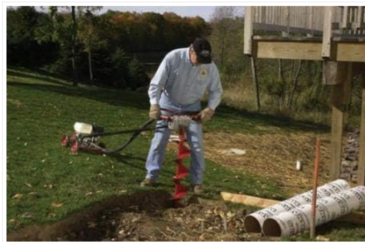
Image: An individual demonstrating the proper technique for operating the Little Beaver Post Hole Digger, maintaining a firm grip and stable stance.
