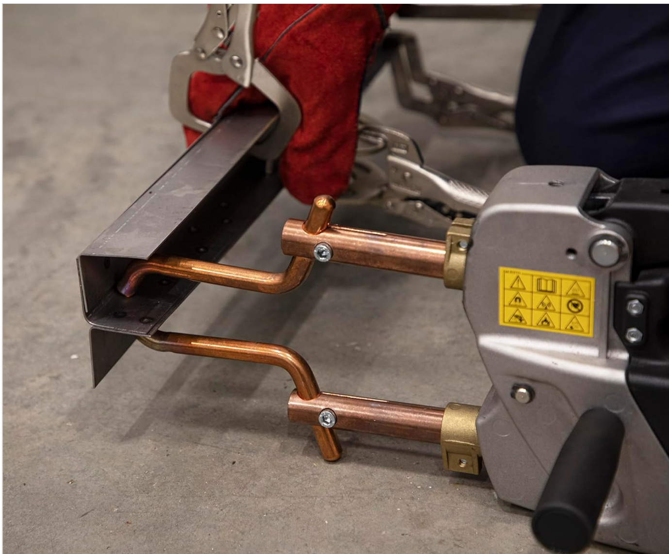
Image 5.2: The spot welder actively joining two metal pieces, demonstrating its application.
