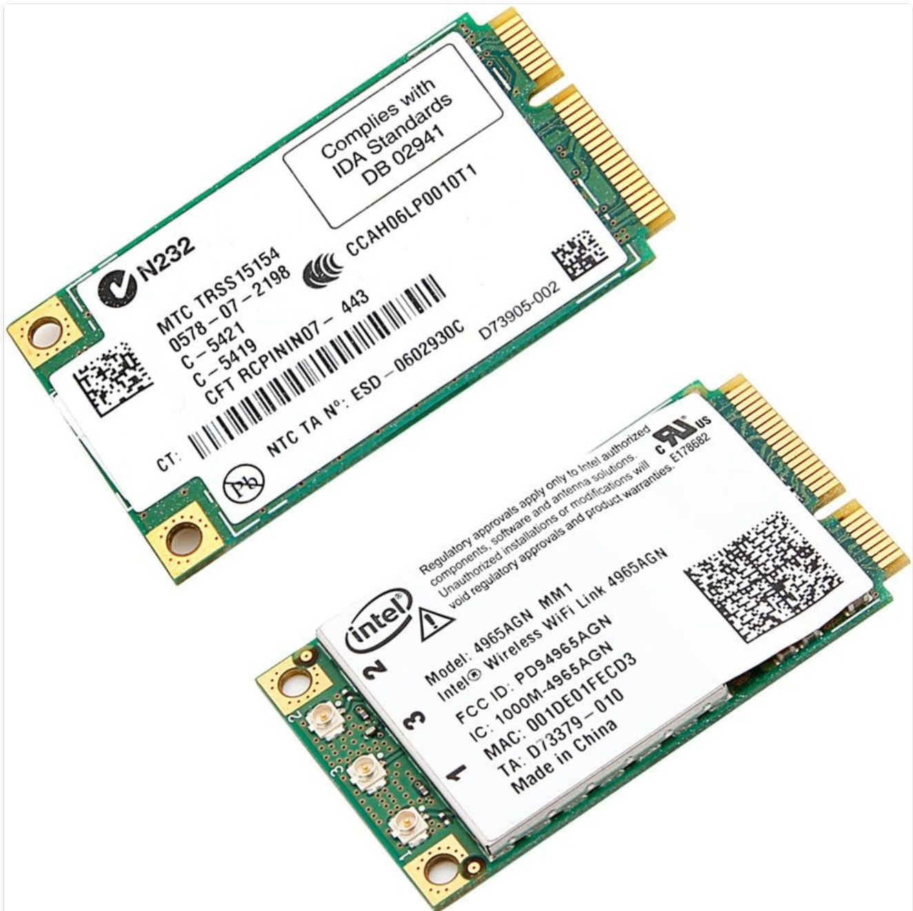
Figure 2: Two Intel 4965AGN adapters, illustrating the top and bottom views. The bottom view clearly shows the antenna connection points (1, 2, 3) and the Intel branding.
