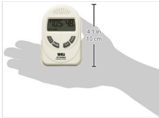
Figure 5.1: The DTH880 unit demonstrating its compact size and the kickstand for desk placement.
