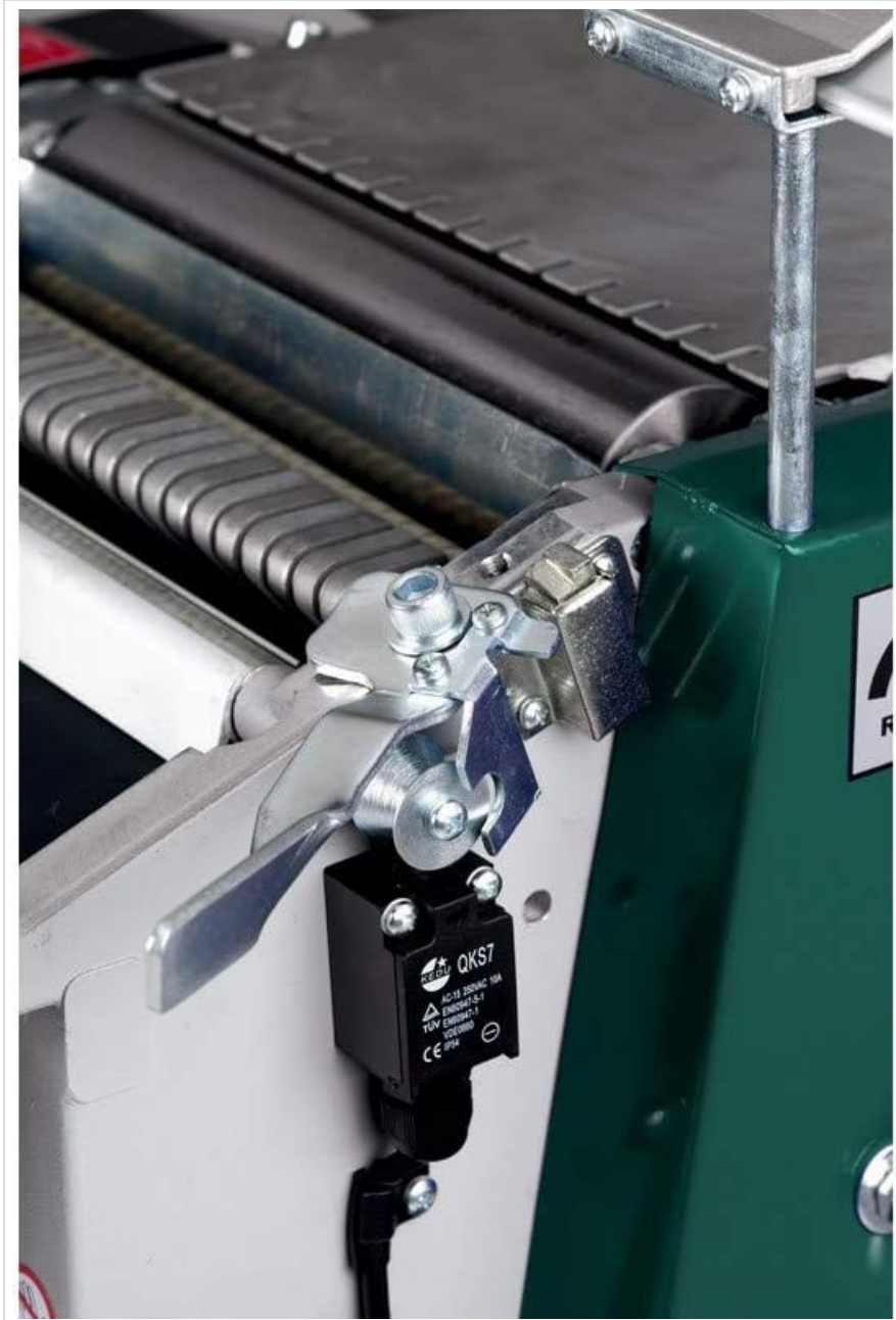
Figure 5.1: Detail of a safety mechanism. This image shows a close-up of a safety switch, which must be properly engaged for the machine to operate.
