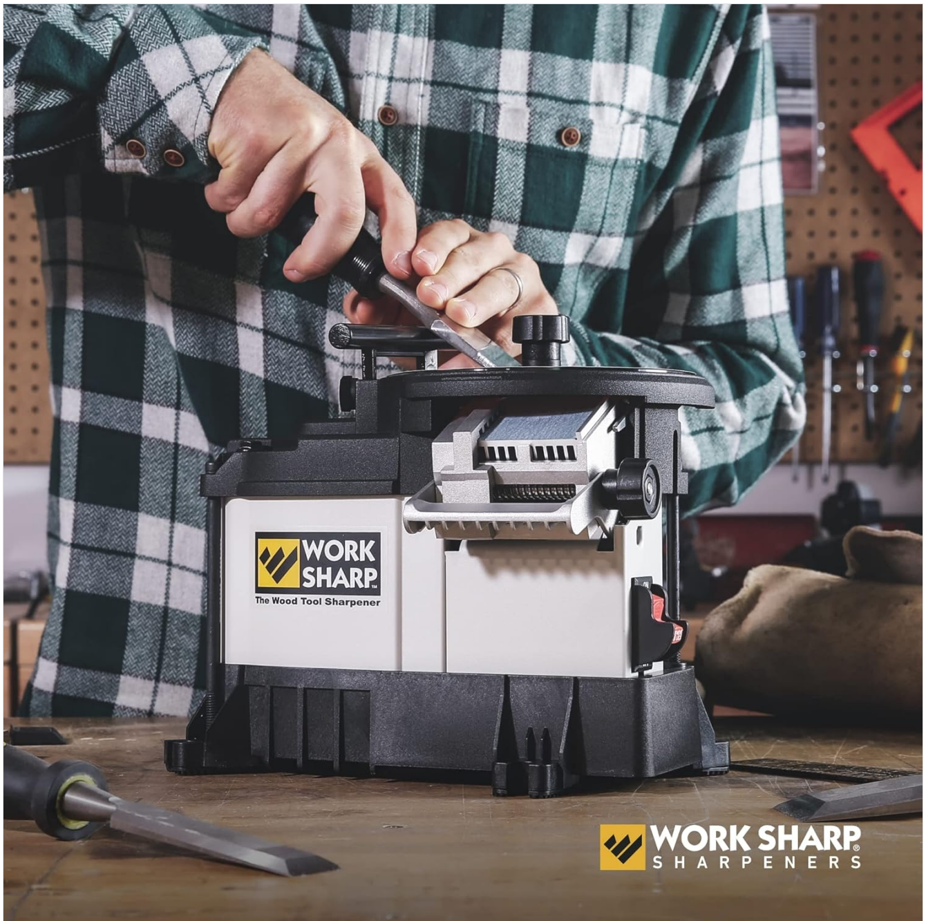
Figure 3.3: Sharpening a carving tool using the slotted Edge-Vision wheel.
