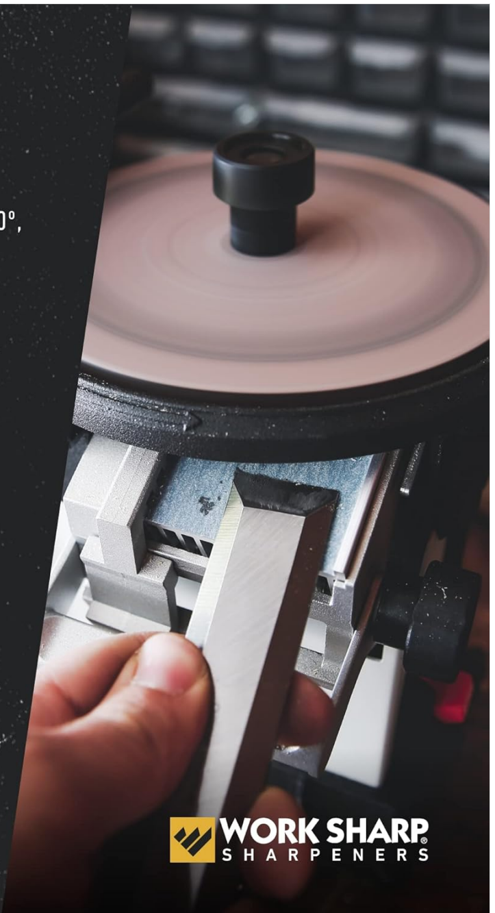
Figure 3.1: Sharpening a chisel using the integrated sharpening port.
