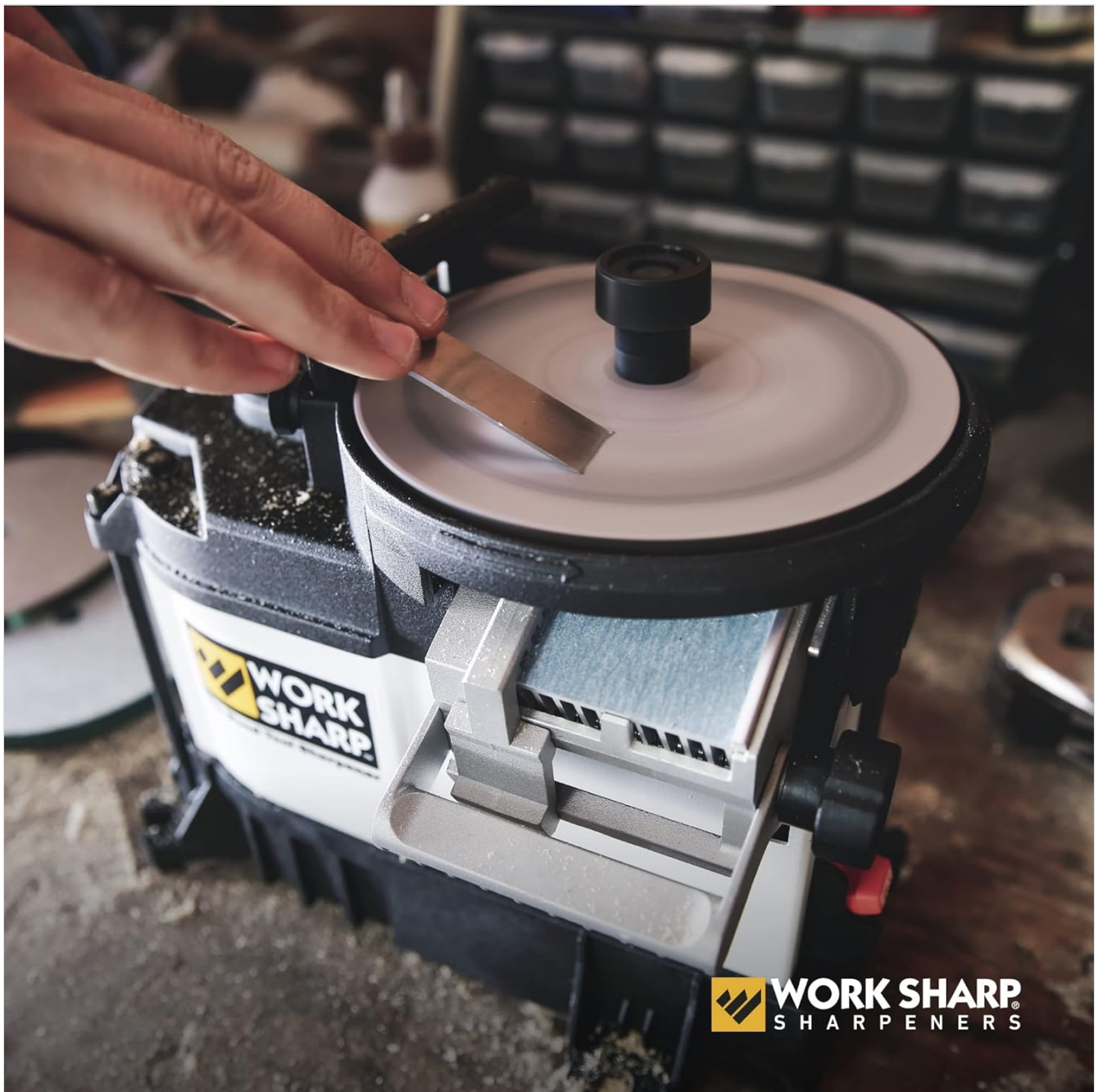
Figure 3.2: Sharpening a plane iron on the top surface of the abrasive disc.
