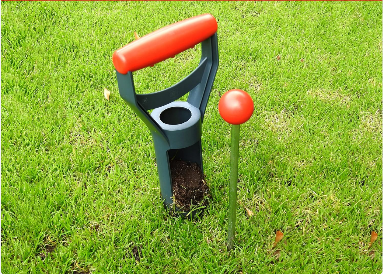
Image: The hole cutter being used to create a precise hole in the ground for trap installation, next to the tunnel probe.
