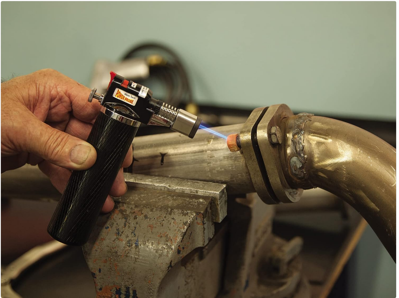
Figure 4: The Micro Torch in action, demonstrating its precision for soldering applications.
