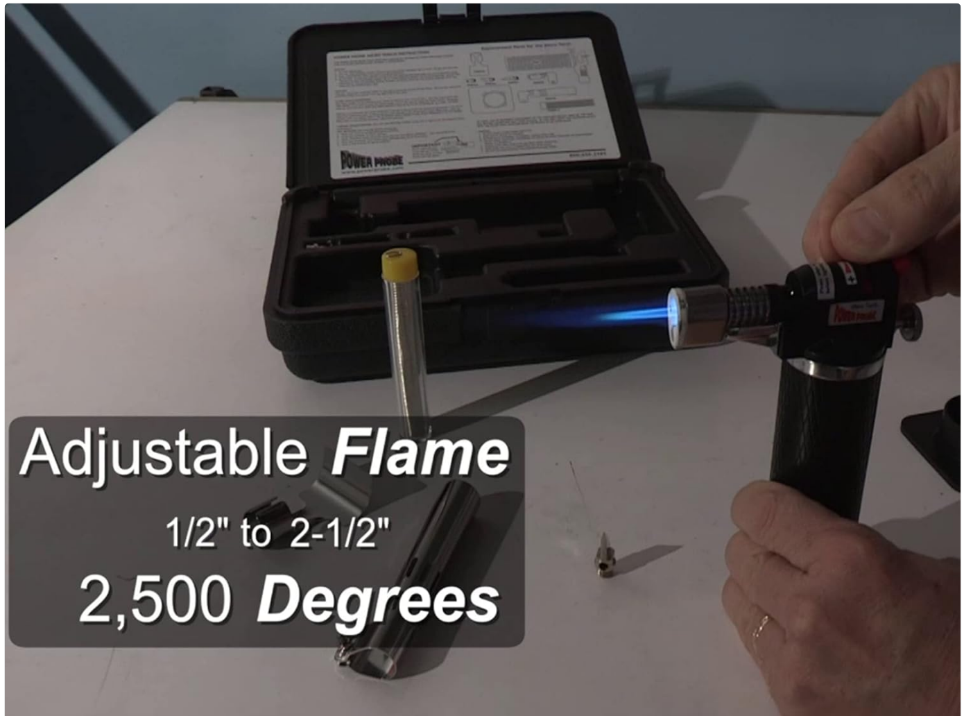
Figure 3: The Micro Torch demonstrating its adjustable flame, capable of reaching up to 2500 degrees Fahrenheit.
