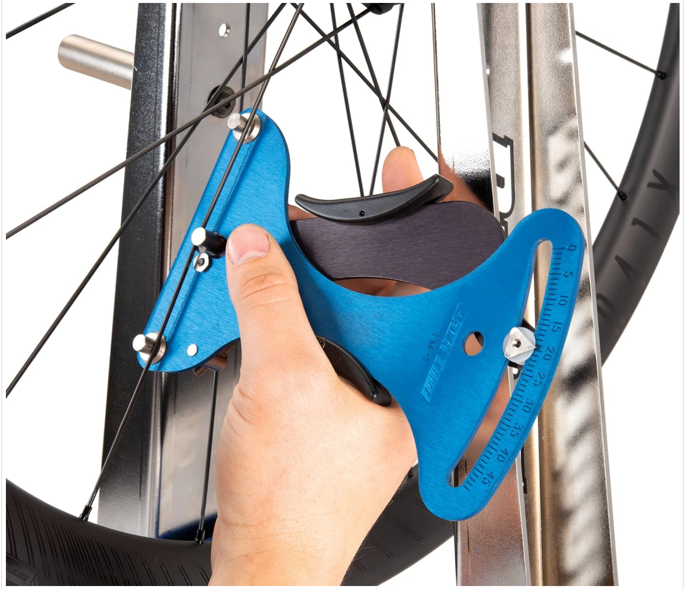
Figure 2: A hand demonstrating the placement of the Park Tool TM-1 on a bicycle wheel spoke for tension measurement.
