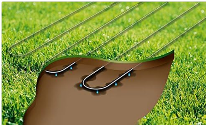
Figure 3: Illustrative diagram of the drip irrigation line installed below ground, showing water delivery to plant roots.
