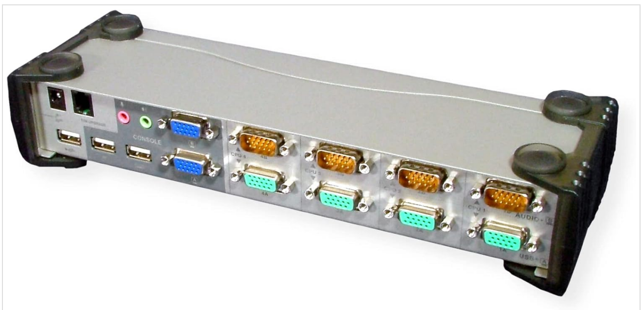
Figure 3.3: Angled Rear View of the ATEN CS1744. This perspective provides a clearer view of the port labels and layout on the rear panel, including the console and CPU connection sections.
