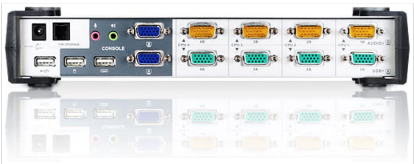
Figure 3.2: Rear Panel of the ATEN CS1744. This image shows the power input, firmware upgrade port, console ports (USB keyboard, USB mouse, audio in/out, dual VGA monitor outputs), and four sets of CPU ports (dual VGA, audio in/out, USB) for connecting to four different computers.
