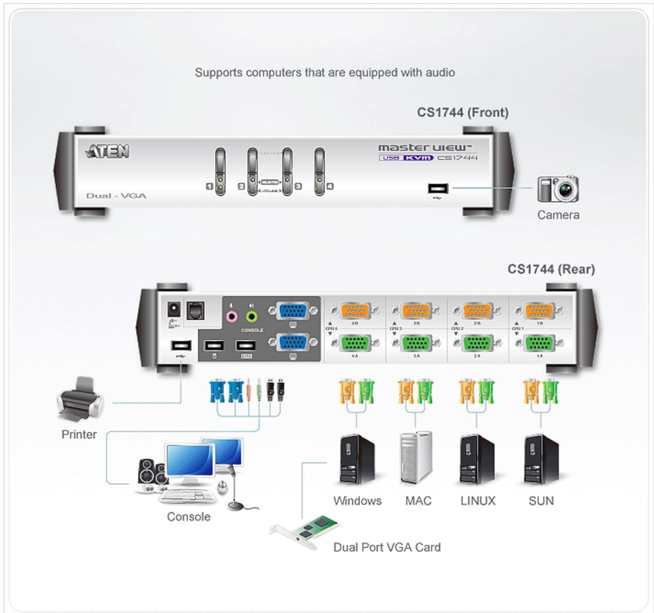
Figure 3.4: Connection Diagram for the ATEN CS1744. This diagram shows the front and rear panels with illustrative connections for a console (keyboard, mouse, dual monitors, speakers, microphone, printer) and four computers (Windows, Mac, Linux, Sun), each with dual VGA outputs, audio, and USB connections to the switch.
