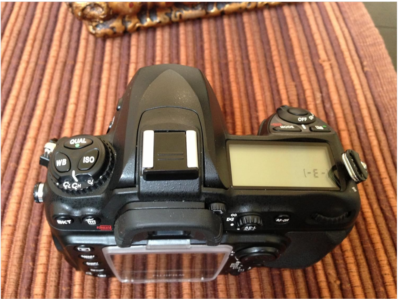
Figure 4.4: Top view of the camera, illustrating the main command dial, shutter release button, and the secondary information display.
