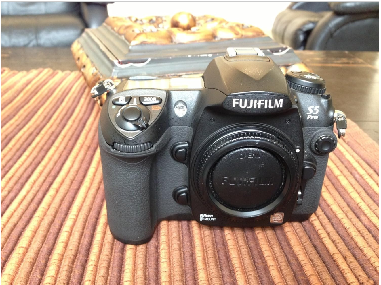
Figure 4.2: Front view of the camera body without a lens, highlighting the Nikon F-Mount for interchangeable lenses.
