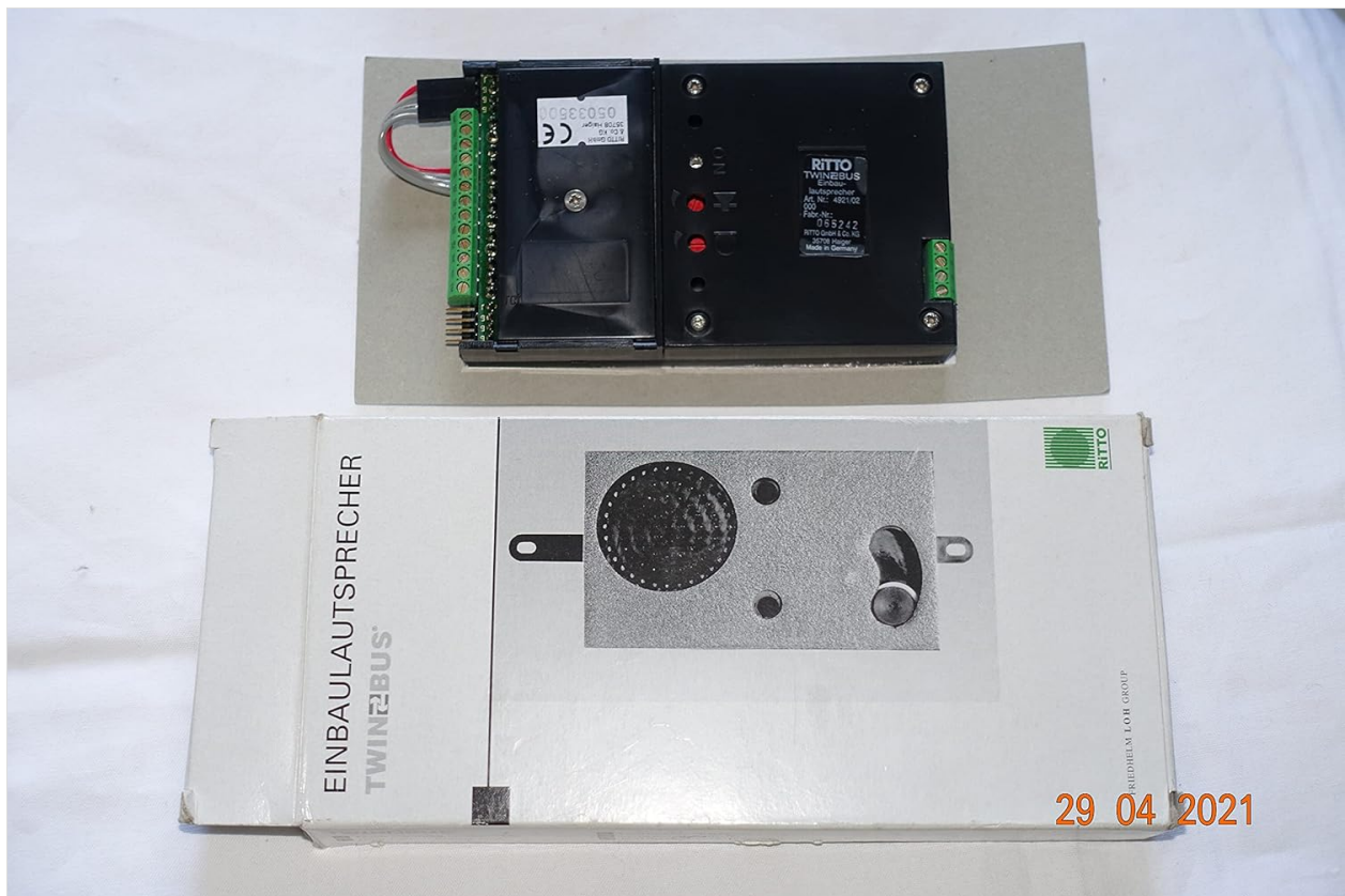
Figure 3.1: Ritto 1492102 Flush Mount Speaker unit and its packaging box.
