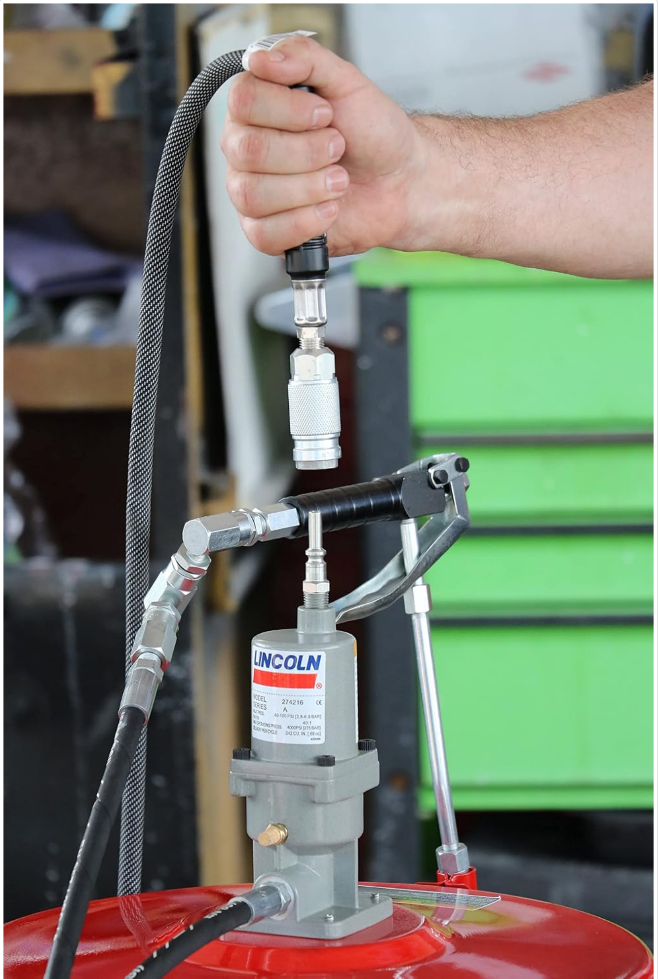
Figure 5: Proper connection of the grease gun to the high-pressure hose.
