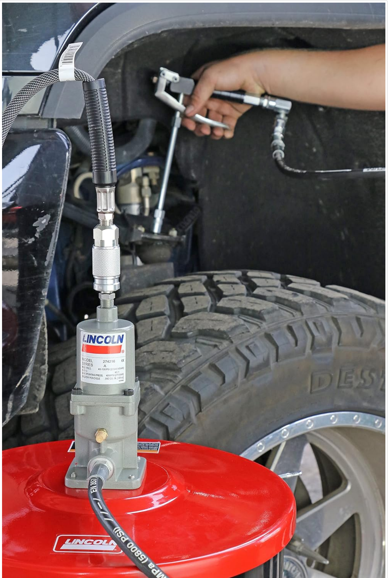
Figure 6: The pump head showing the air regulator and pressure gauge.
