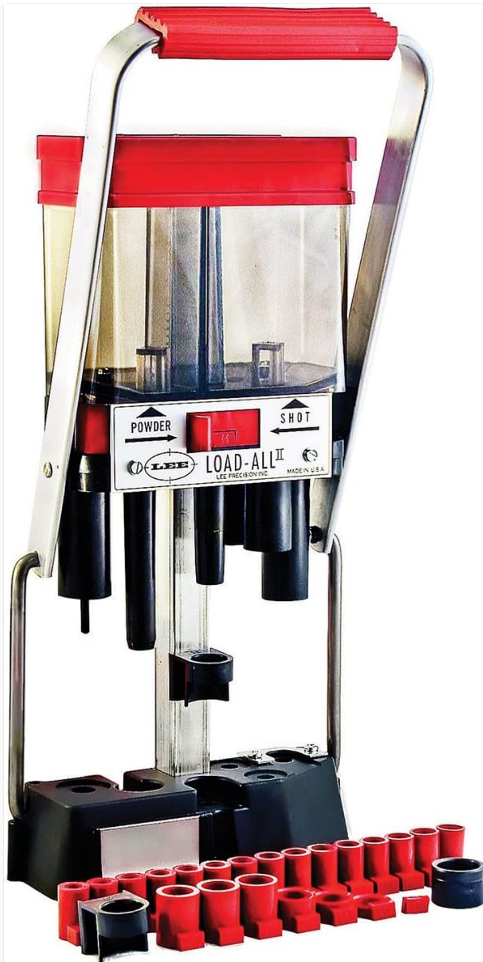
Figure 1: Front view of the Lee Precision II Shotshell Reloading Press, showcasing its compact design and integrated powder and shot hoppers.
