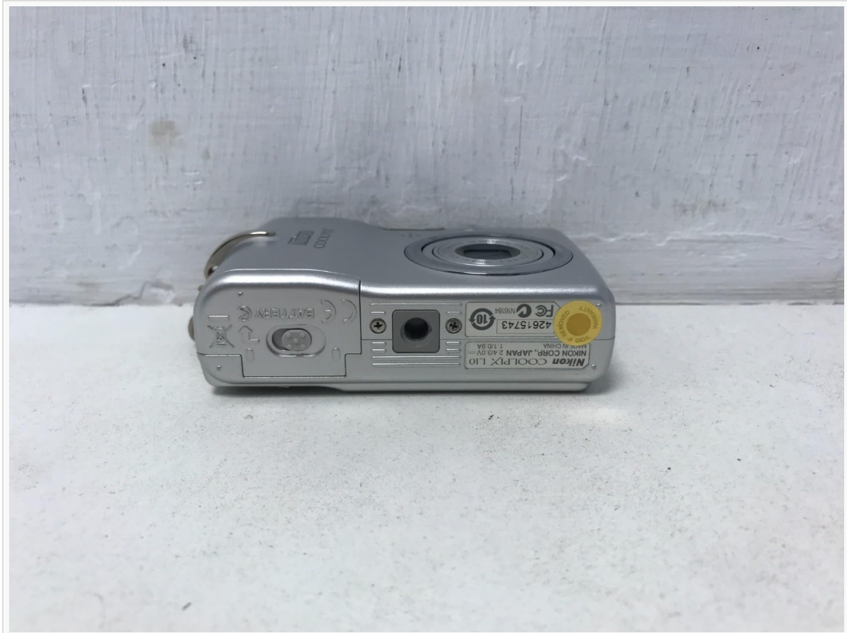
Figure 5: Battery Compartment. The bottom of the camera showing the battery compartment latch and tripod socket.
