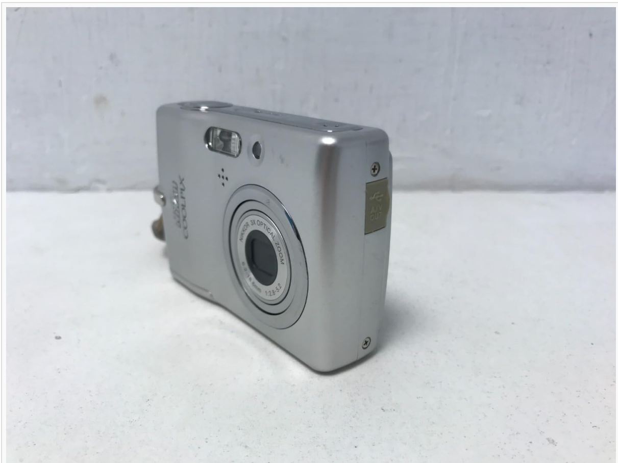
Figure 4: Side View. The side of the camera features the AV OUT port, used for connecting to a television or computer.
