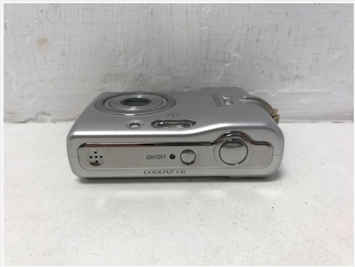
Figure 3: Top View. This image highlights the power button and shutter release button located on the top of the camera.
