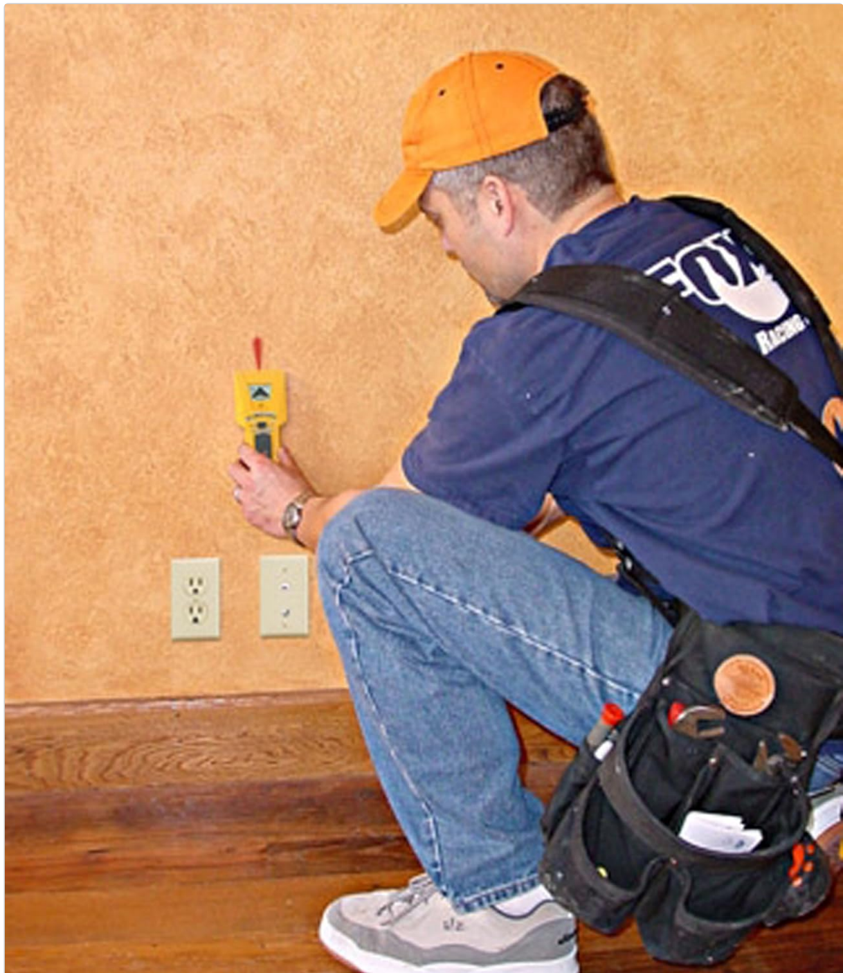
Figure 3: A user operating the Zircon StudSensor Pro LCD on a wall to locate studs.
