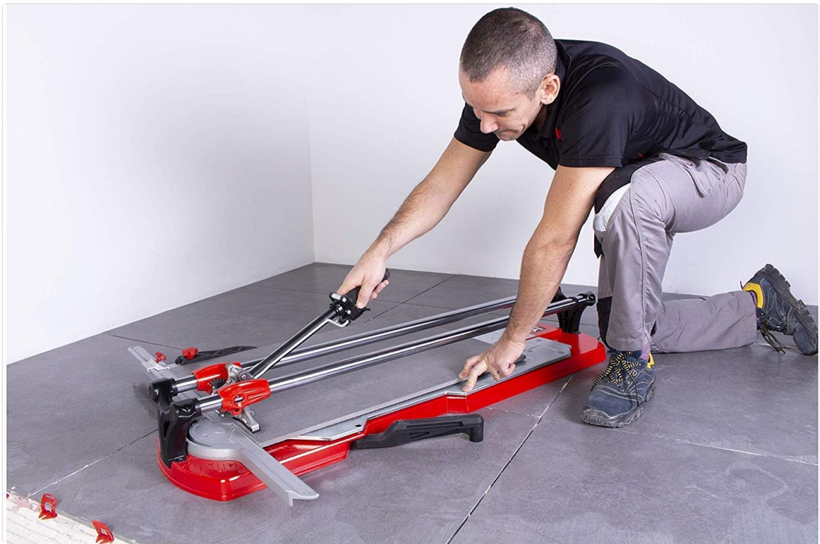
Figure 4: A user carefully positioning a large format tile on the cutter, aligning the cut line with the scoring guide.
