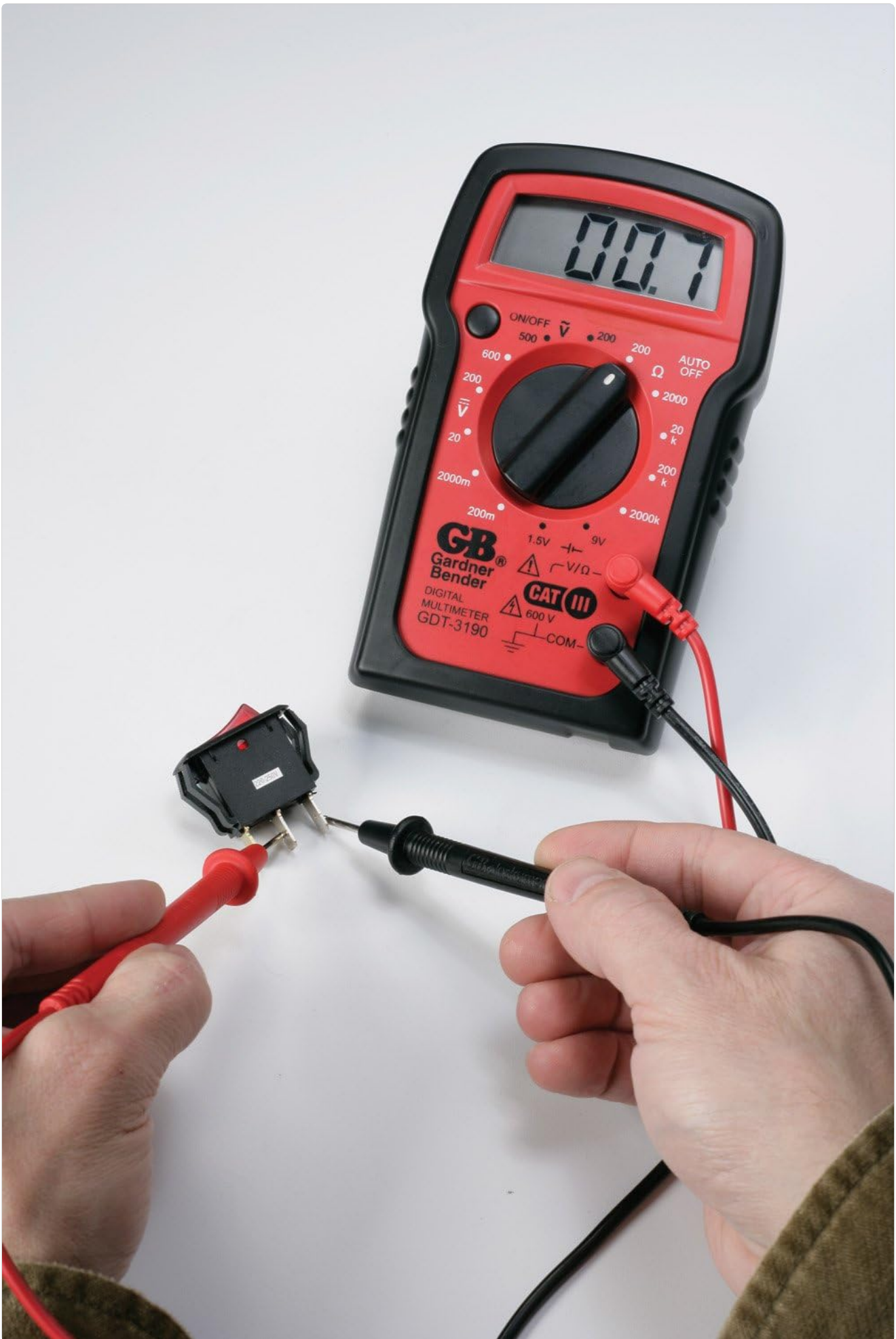
Figure 3.2: Testing a switch for continuity or resistance using the multimeter's probes.
