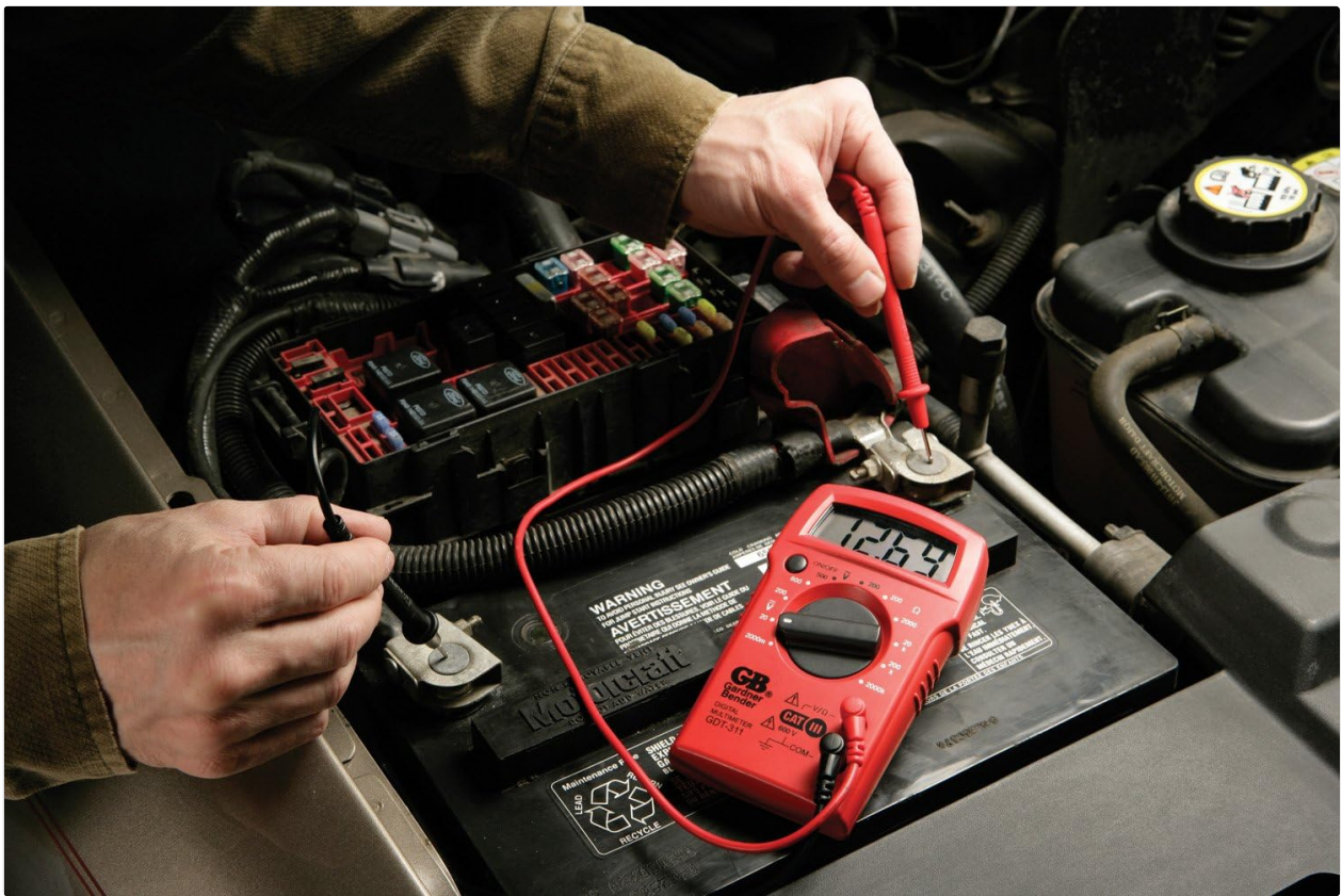
Figure 3: The GDT-311 Multimeter in use, measuring the voltage of a car battery. The digital display clearly shows the reading.
