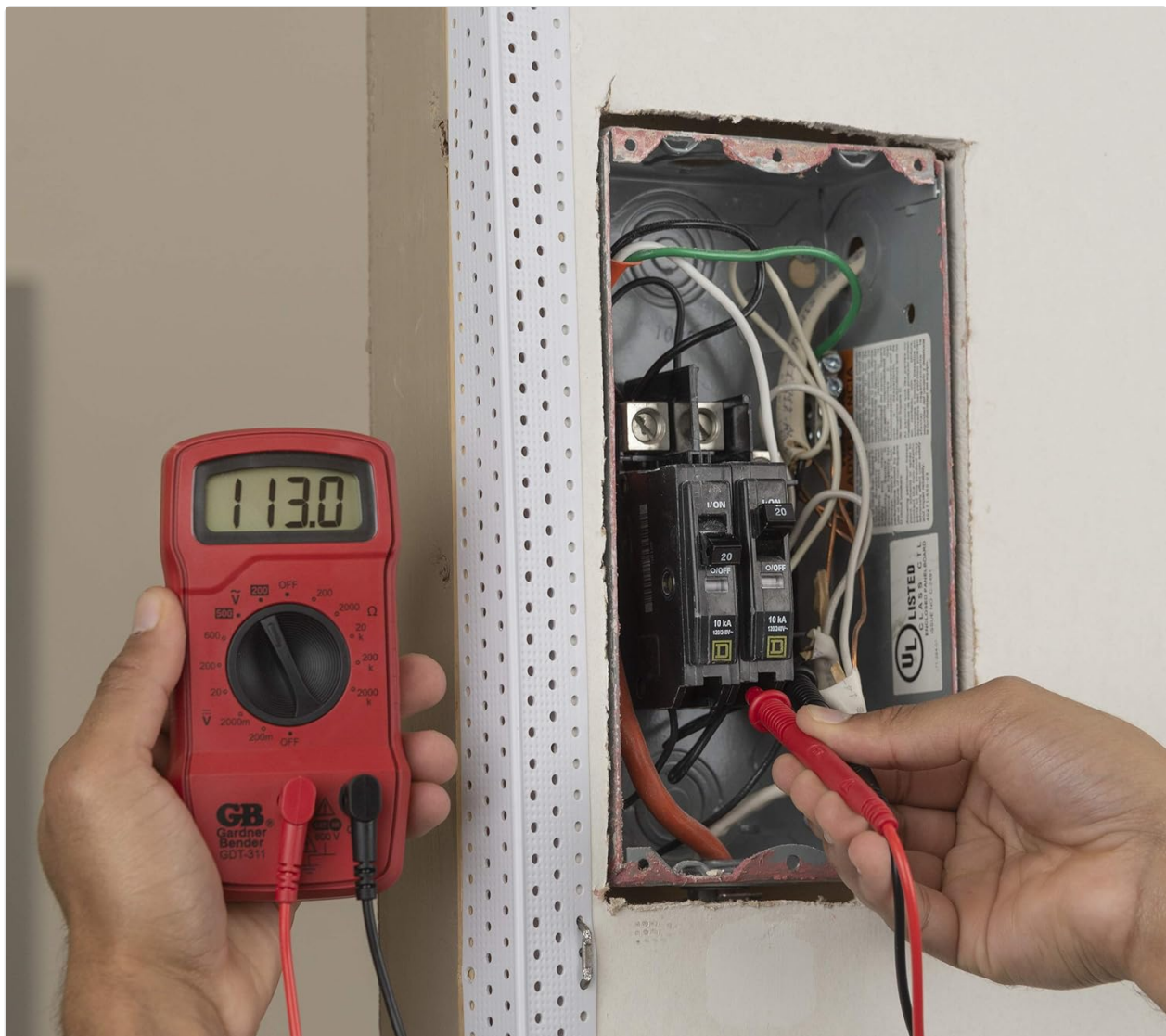
Figure 5: The GDT-311 Multimeter in action, testing a circuit breaker panel. The display shows the measured voltage, indicating its utility for electrical diagnostics.
