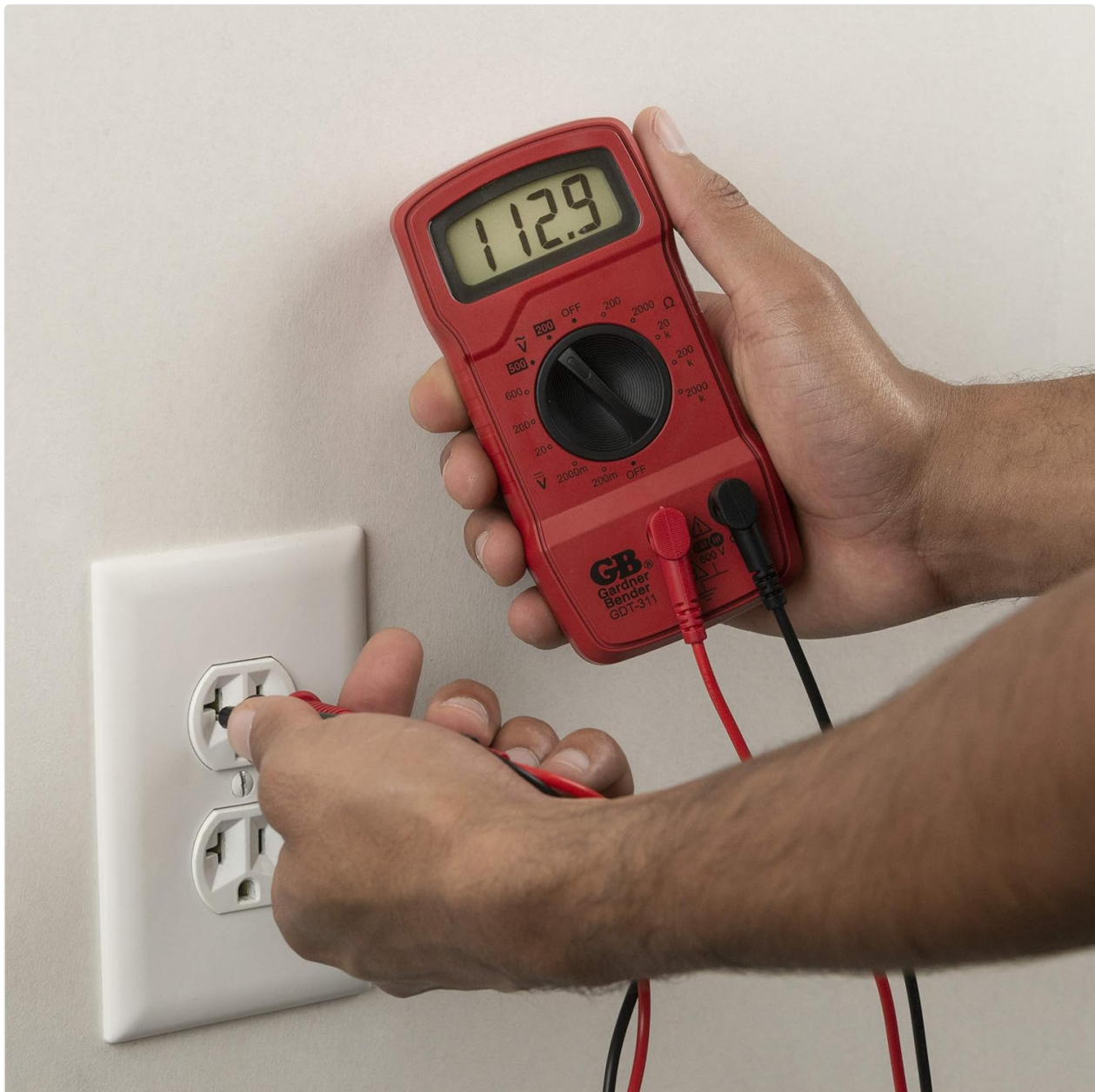
Figure 4: The GDT-311 Multimeter being used to test an AC wall outlet, demonstrating its capability to measure alternating current voltage.
