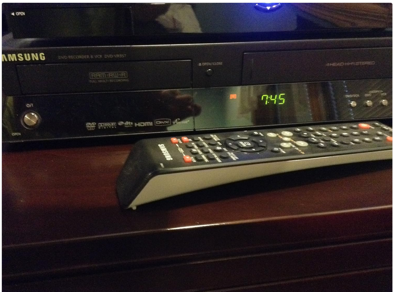
Image 1: Front view of the Samsung DVD-VR357 unit with its remote control. The unit features a DVD tray on the left, a VCR slot on the right, and a central display showing "7:45". Below the display are various control buttons and indicators, including power, open/close, and input selection. The remote control is positioned in front of the unit.
