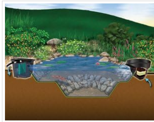
Image: Cross-section diagram illustrating the ecosystem approach of an Aquascape pond, showing skimmer, BioFalls, and pond shelves.
