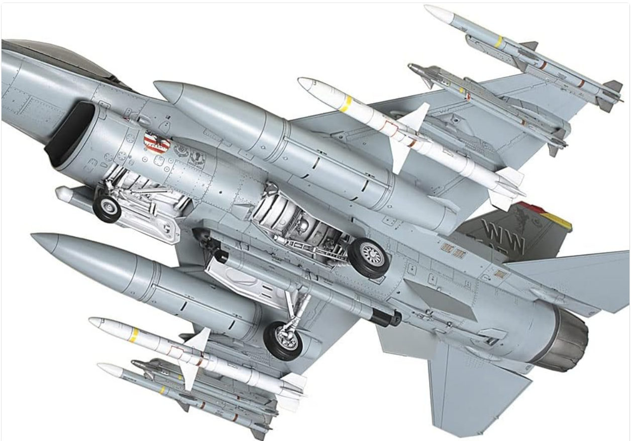
Figure 3.5: The underside of the F-16CJ model, showcasing the detailed landing gear and the array of weapons and external fuel tanks.
