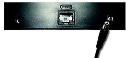
Figure 4-2: Connect the Power
