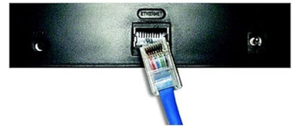
Figure 4-1: Connect the Ethernet Cable
