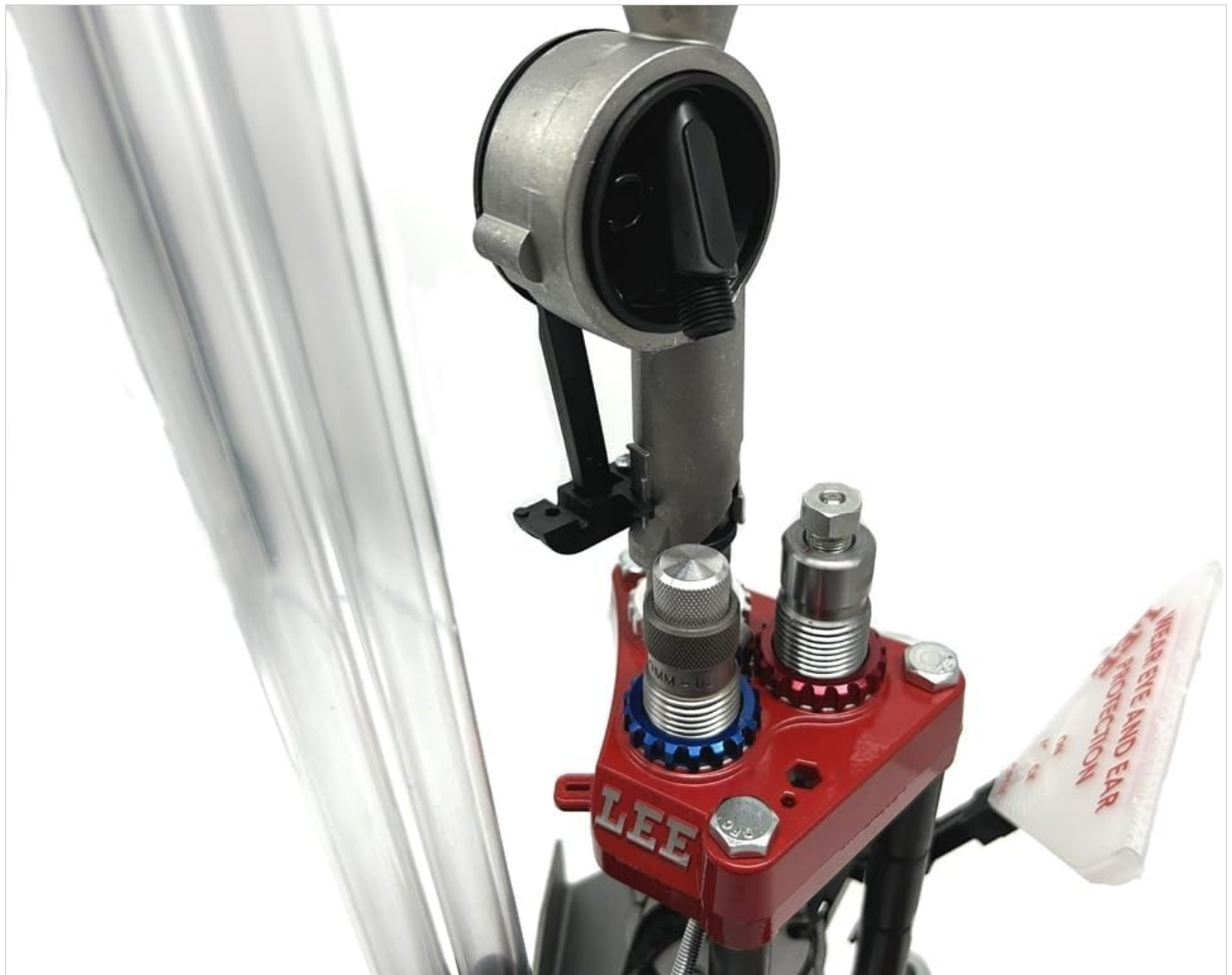
Figure 1: Close-up of the die stations and powder measure assembly.
