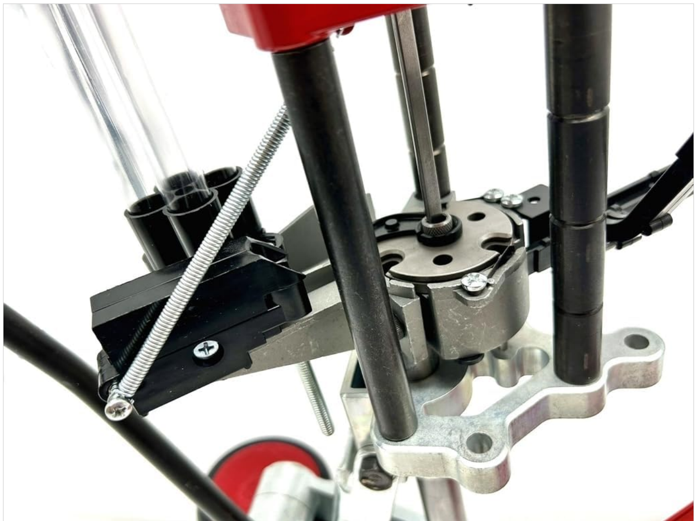
Figure 2: View of the shell plate and primer feed mechanism.
