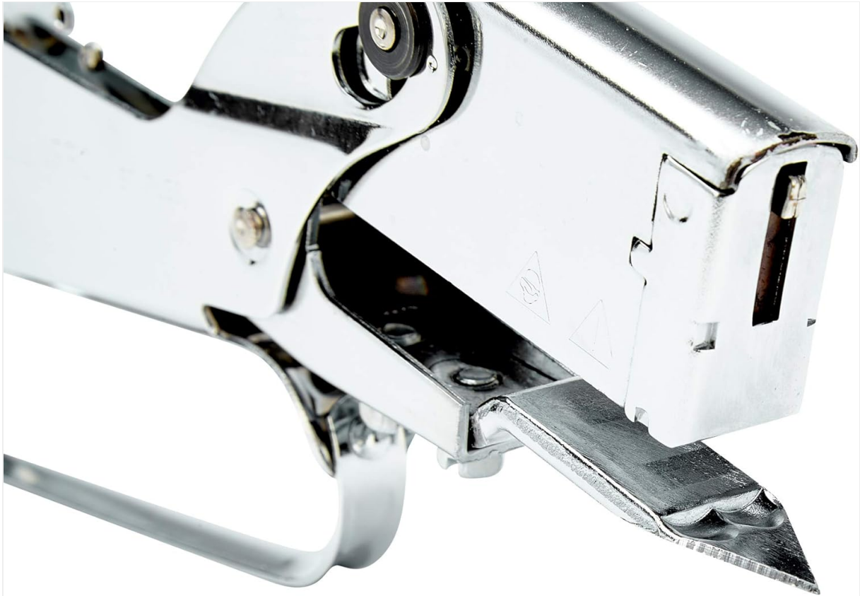
Figure 2: Close-up view of the spear-pointed nose, essential for piercing materials before stapling.
