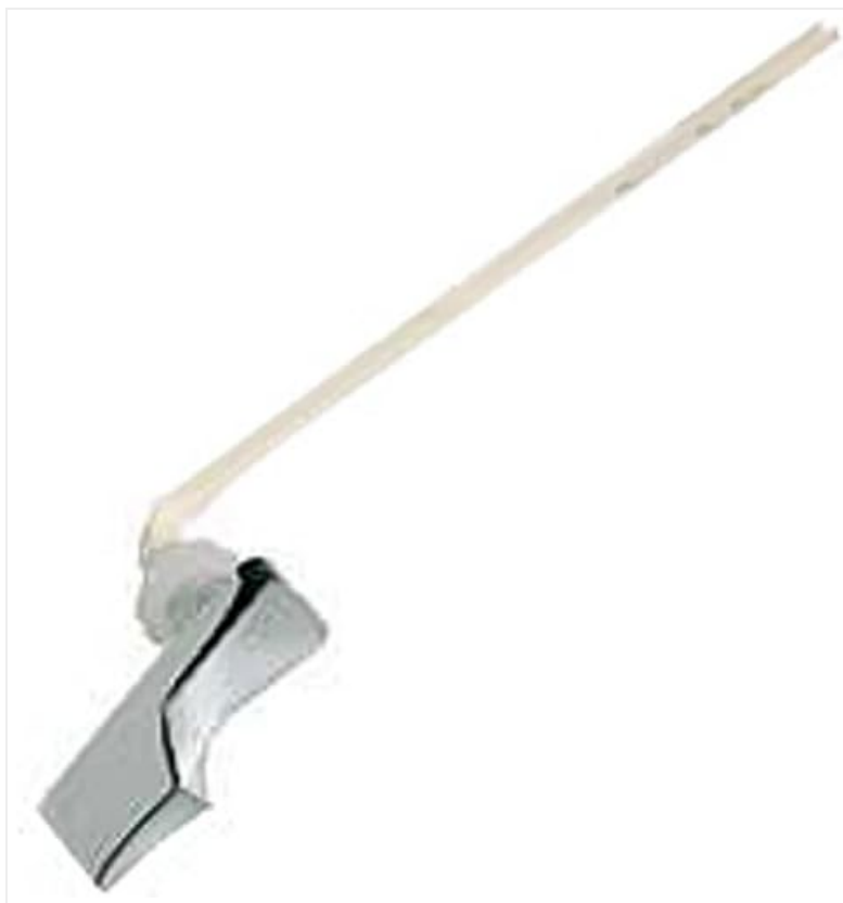
Image: Illustrates the Danco tank lever with its long plastic arm, indicating where it can be trimmed to fit different tank depths. The arm is designed with markings for 4, 6, 8, and 10-inch lengths.
