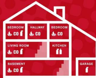
Image 4.1: Recommended Smoke Alarm Placement. This diagram illustrates ideal locations for smoke alarms, carbon monoxide alarms, and fire extinguishers throughout a typical home, including bedrooms, hallways, living room, kitchen, basement, and garage.
