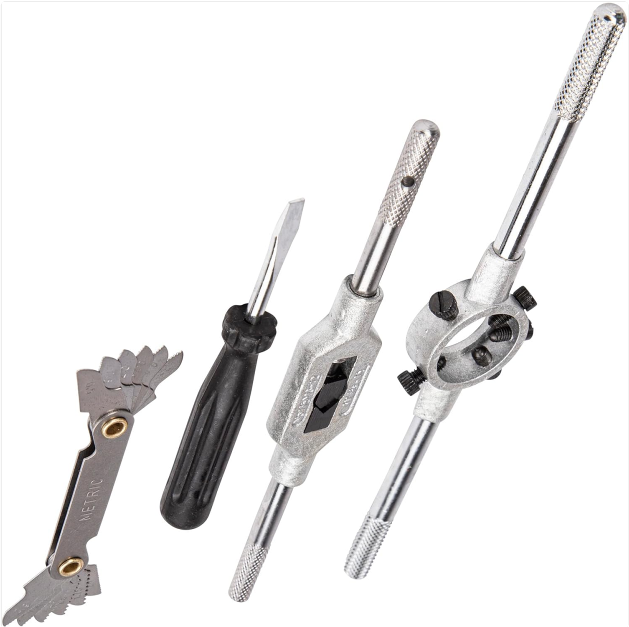
Figure 2.2: Key accessory tools: thread gauge, screwdriver, tap wrench, and die stock.
