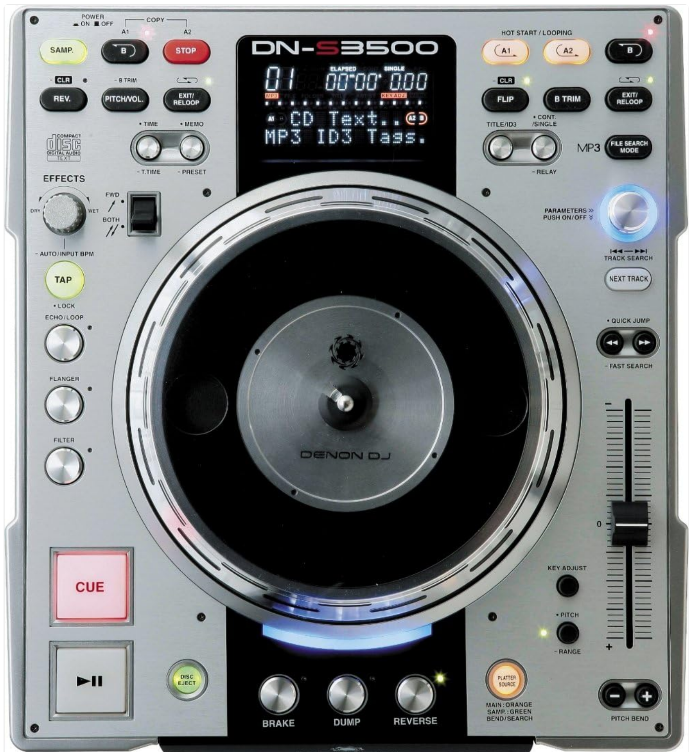
Figure 4: Detailed view of the Denon DNS3500's motorized platter and adjacent controls for effects and pitch adjustment.
