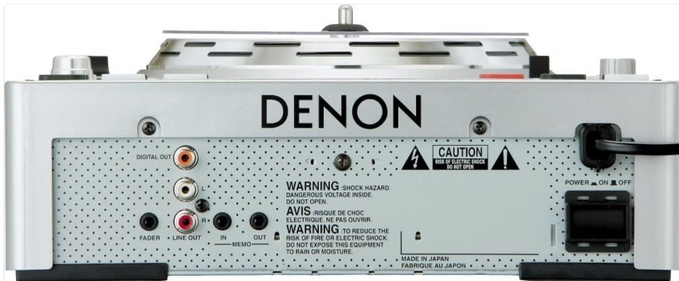
Figure 2: Close-up of the Denon DNS3500 rear panel, highlighting the power switch and safety warnings.
