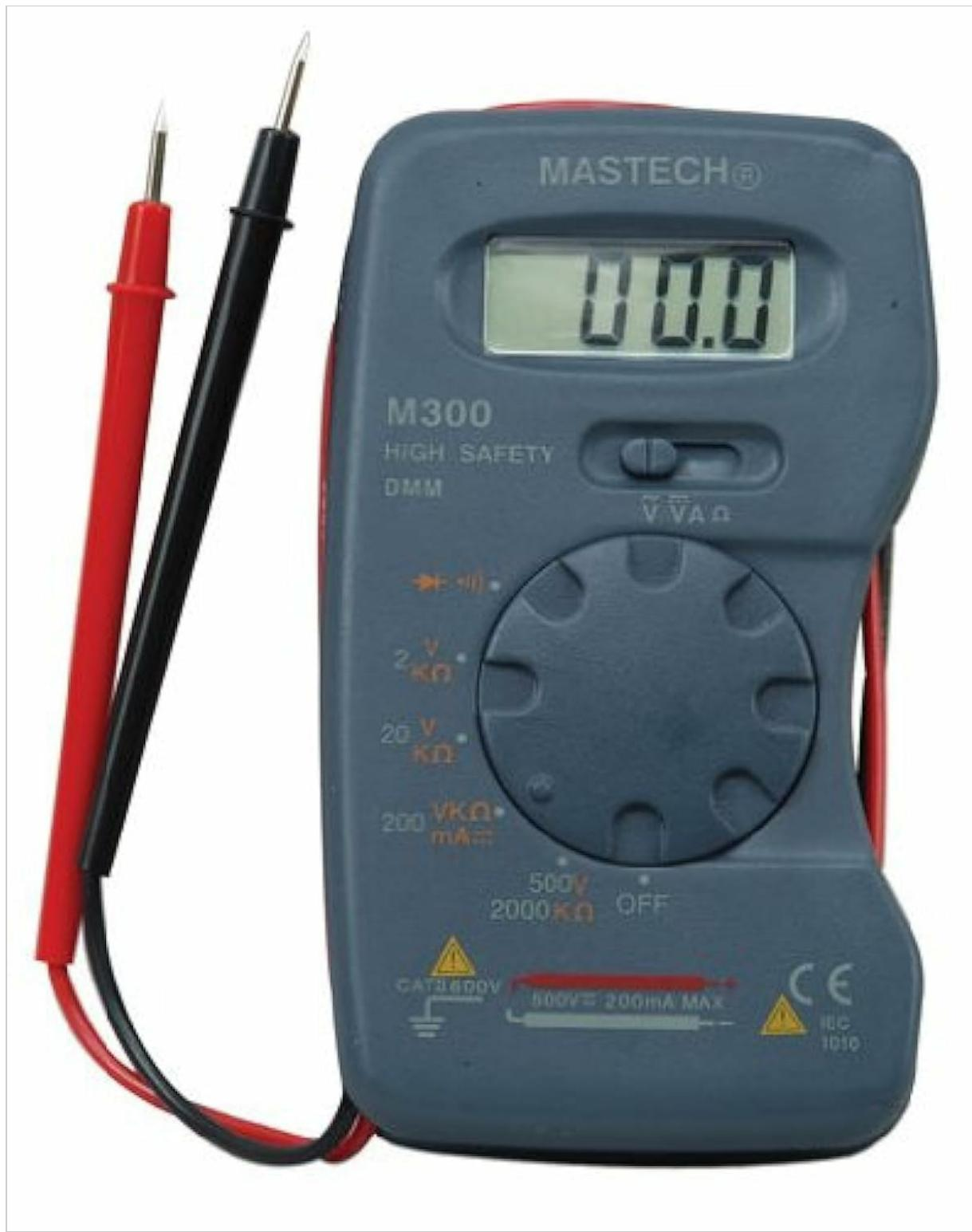
Figure 3.1: Front view of the Mastech M300 Mini Digital Multimeter, showing the LCD display, rotary switch, function buttons, and integrated red and black test leads.
