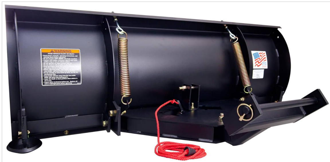
Figure 4.2: Rear view of the plow blade, illustrating the spring mechanism and angle adjustment system.
